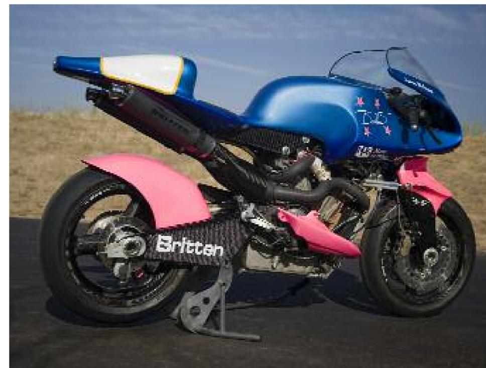
John Britten experimented with different handmade exhaust routings, and Virgil Elings' bike features a less convoluted version.
