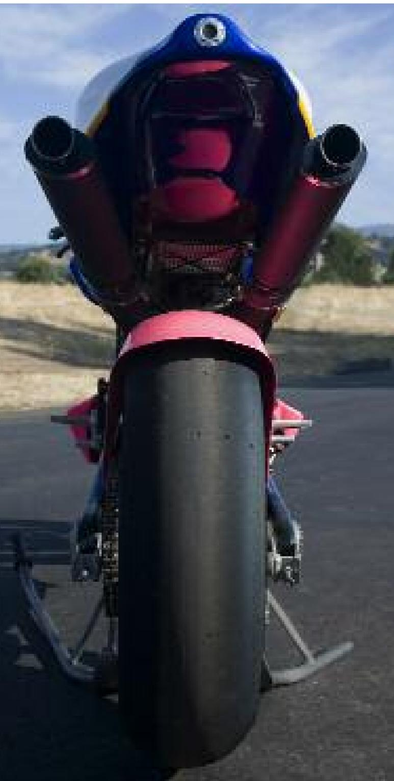
The V-1000's aluminum exhaust silencers produce a deep but muted bass sound, and its underseat radiator is notorious for heating up the thin seat.
